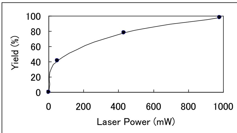
Figure 4. Laser power dependence of the yield of Product **2** in photolysis of Compound **1** in  $\text{CDCl}_3$ . Exposure time was 60 minutes.
