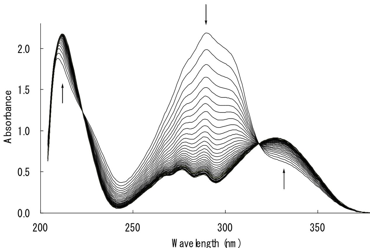
Figure 2. Change in absorption spectra of compound 1 ( $3.0 \times 10^{-4}$  M) in MeOH after photoirradiation for 15 seconds using a 300 W Xe lamp (Pyrex filter)
