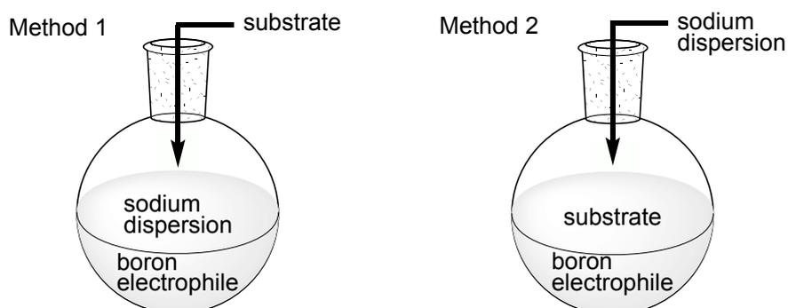
Figure 1. Two extreme methods to treat a substrate with sodium dispersion
