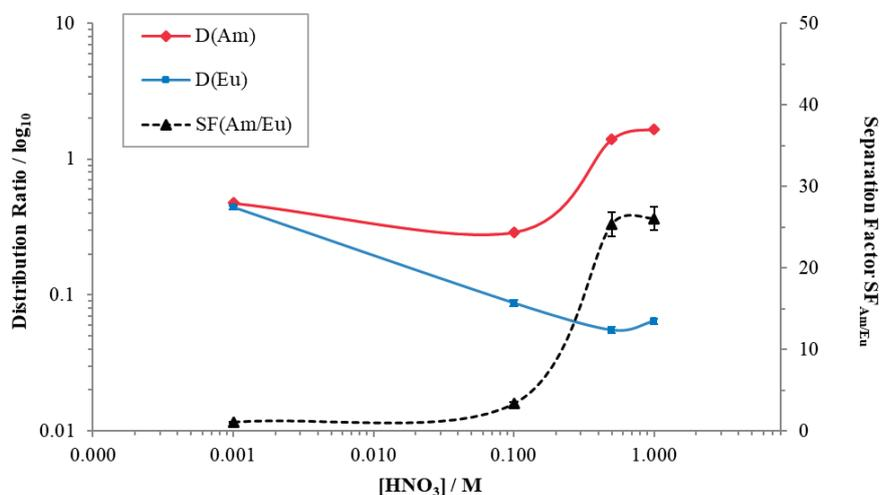
**Figure 3.** Extraction of Am(III) and Eu(III) by 10 mM tetra(4-hydroxyphenyl)BTPhen **3** in cyclohexanone as a function of nitric acid concentration. The system was shaken for 90 mins at 1800 rpm.
