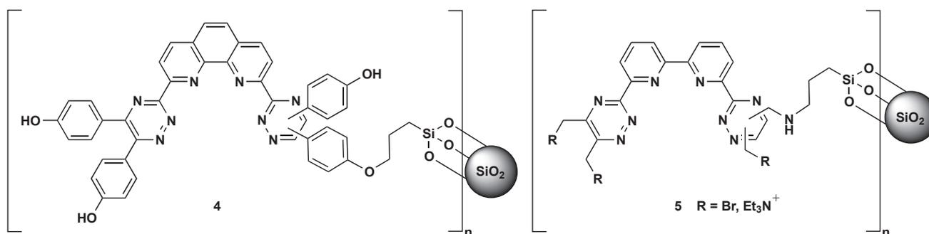
**Figure 2.** Structures of tetra(4-hydroxyphenyl)BTPhen-functionalized silica gel **4** and tetra-bromomethylBTBP-functionalized silica gel **5**
