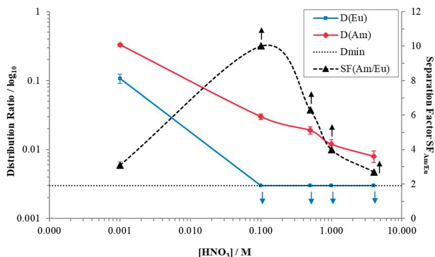
**Figure 4.** Extraction of Am(III) and Eu(III) by 5 mM tetra(4-hydroxyphenyl)BTPhen **3** in octanol as a function of nitric acid concentration. The system was shaken for 90 mins at 1800 rpm.
