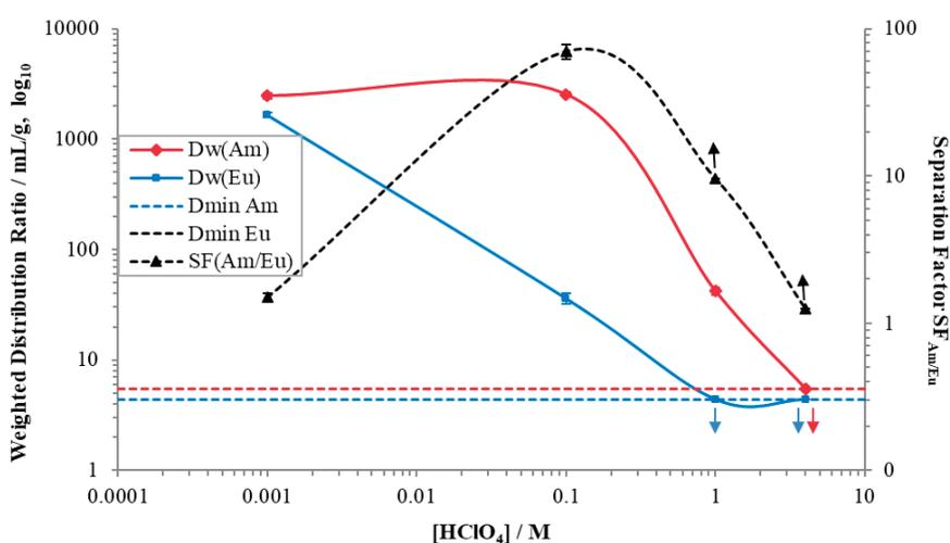
**Figure 7.** Extraction of Am(III) from Eu(III) by 6.4 mg of silica immobilized tetra(4-hydroxyphenyl)BTPhen **4** as a function of perchloric acid concentration.  $V/m = 143 \text{ mLg}^{-1}$ . The system was shaken for 90 mins at 1800 rpm.
