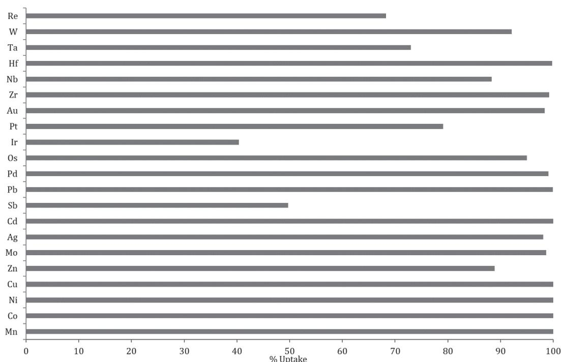
**Figure 8.** Percentage uptake of metal ions (10 ppb) from aqueous solution at pH 0.5 (HNO<sub>3</sub>) by tetra(4-hydroxyphenyl)BTPhen functionalized silica 4
